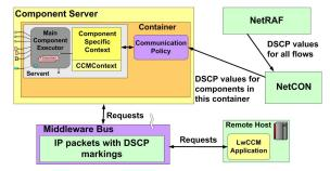
Figure 5: NetCON's Container Auto-configurations
