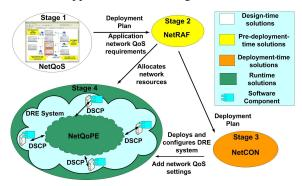
Figure 1: NetQoPE's Four-stage Architecture
